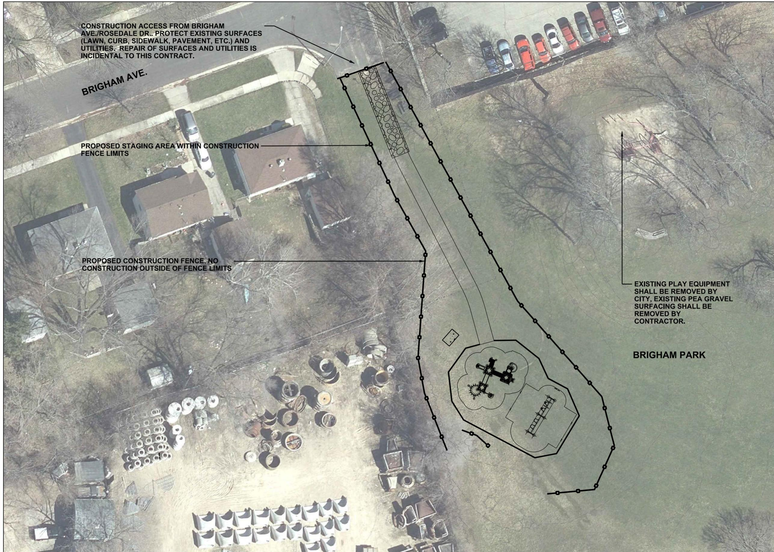
CONSTRUCTION ACCESS FROM BRIGHAM AVE./ROSEDALE DR.. PROTECT EXISTING SURFACES (LAWN, CURB, SIDEWALK, PAVEMENT, ETC.) AND UTILITIES. REPAIR OF SURFACES AND UTILITIES IS INCIDENTAL TO THIS CONTRACT.
